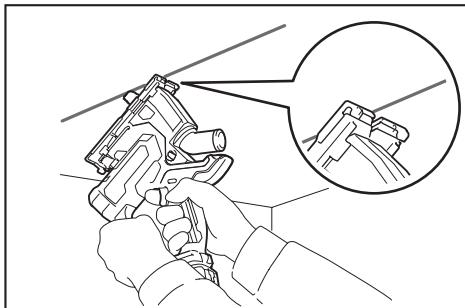
2. Slowly pull the trigger without the blade making any contact with the workpiece. When the blade attains full speed, push the tool toward the workpiece. As the blade pierces the workpiece, make the whole surface of the base cover contact with the workpiece.
