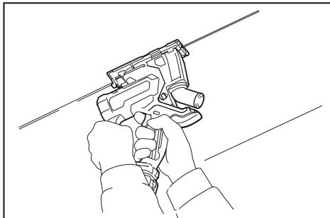
3. Move the tool straight forward until the cutting finishes.
